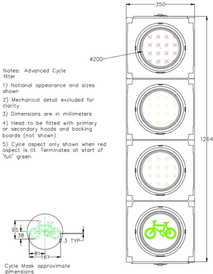
Figure 1 - Advanced Green Cycle Filter
